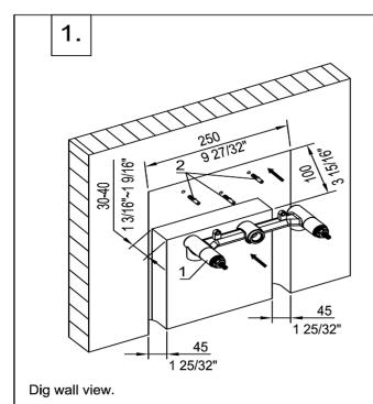
1.Measure the positions of the 3-Ø6 holes in the wall space of pre-digged, knock the expansion plugs(2) into the holes.
